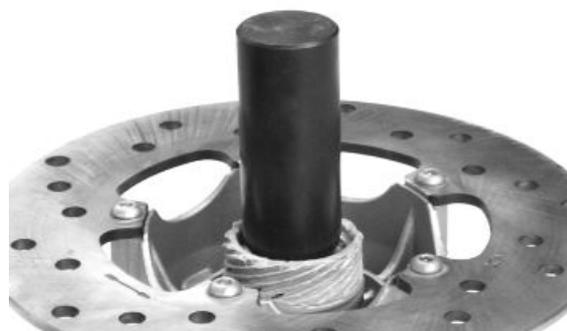
Soap-based lithium grease with NLGI 3; ISO-L-XBCHA3, DIN K3K-20
