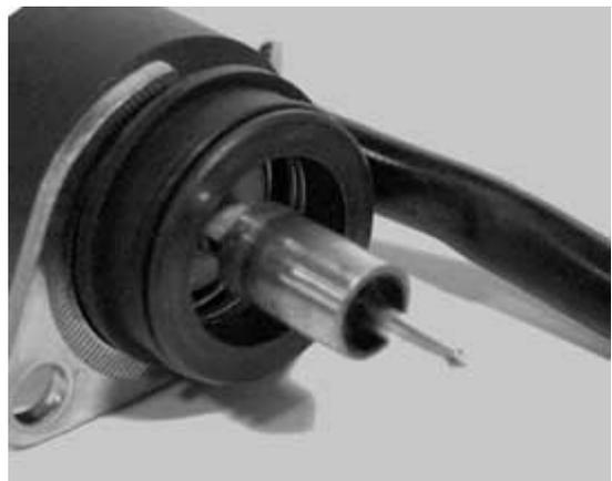
With a 12V battery power the automatic starter and check that the piston protrudes as much as possible.
